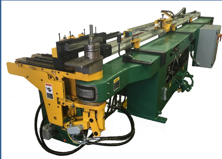
Pines® Model 1 Extrusion Bender with 18' Carriage Travel
