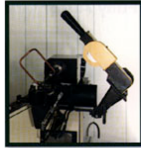
Heavy Duty Head handles up to .250 O.D.
